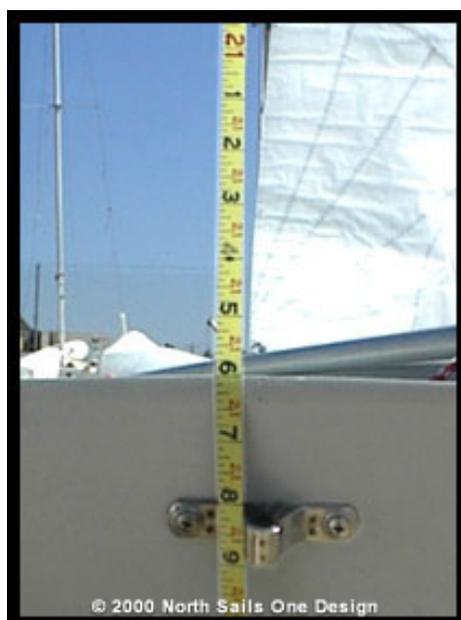
Figure 3 - Mast rake measured to intersection of transom and aft deck.
